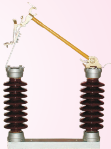
22/33 KV Outdoor Expulsion type Drop Out Fuse Solidcore Insulators with channel Base. Test as per IS-9385/1983
